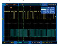
Beneficial for applications such as  $1^2$ C serial data streams, deep memory lets you capture waveforms in high resolution while maintaining a high sample rate over a longer period of time. Up to 2.4 Mpts of memory can be captured in as fast as 5 seconds\* using binary transfer through the LAN or USB interface.
