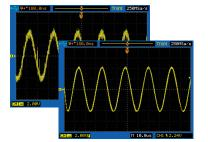
Filter out unwanted signal components such as various types of noise with built-in digital filters. Choose from Low-Pass, High-Pass, Band-Pass, and Band-Stop filters.
