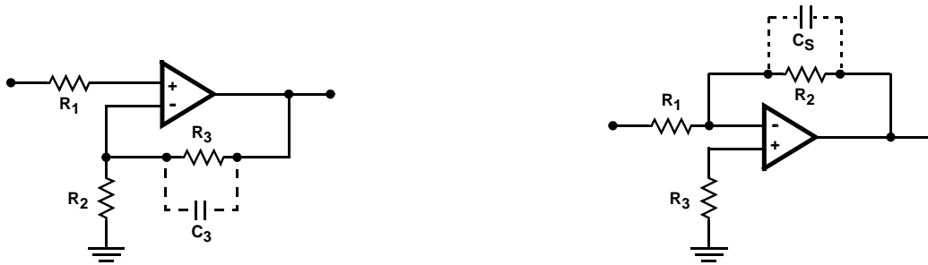
FIGURE 3. SUGGESTED OFFSET VOLTAGE ADJUSTMENT
