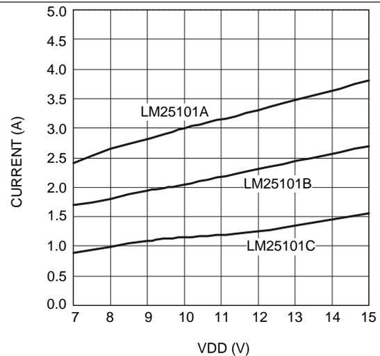
Figure 3. Peak Sinking Current vs Supply Voltage
