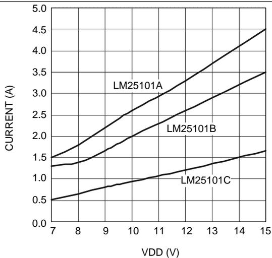
Figure 2. Peak Sourcing Current vs Supply Voltage
