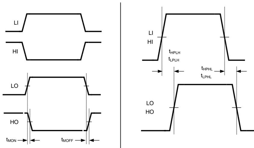
**Figure 1. Timing Diagram**
