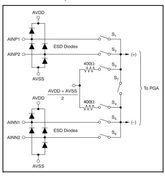
Figure 26. Analog Inputs and Multiplexer
