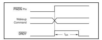
Figure 50. PWDN Pin and Wake-Up Command Timing (Table 12 Shows t<sub>DR</sub>)
