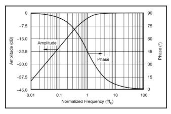
Figure 46. HPF Amplitude and Phase Response
