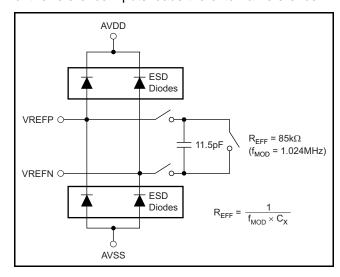
Figure 36. Simplified Reference Input Circuit
