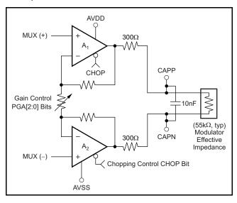
Figure 29. PGA Block Diagram
