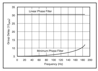
Figure 44. FIR Group Delay (f<sub>DATA</sub> = 500Hz)
