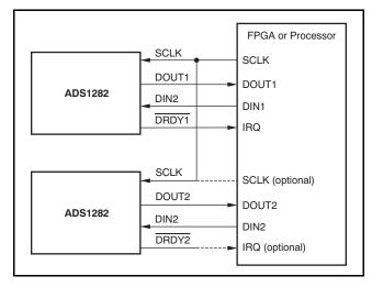
Figure 53. Interface for Multiple Devices
