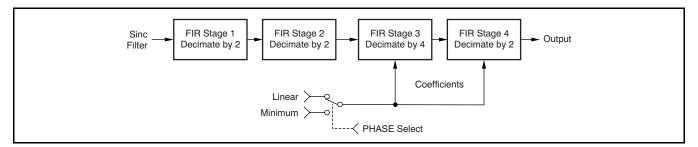
Figure 40. FIR Filter Sub-Stages
