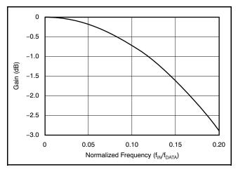
Figure 39. Sinc Filter Roll-Off
