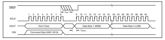
Figure 57. Read Data by Command, RDATA (t<sub>DDPD</sub> Timing is Given in Table 14)
