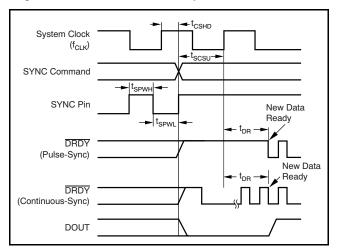
Figure 47. Pulse-Sync Timing, Continuous-Sync Timing with Single Sync
