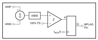
Figure 33. Modulator Over-Range Block Diagram
