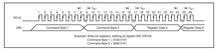
Figure 64. Write Register Data (Table 21 Shows t<sub>DLY</sub>)
