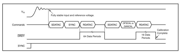
Figure 60. Offset and Gain Calibration Timing
