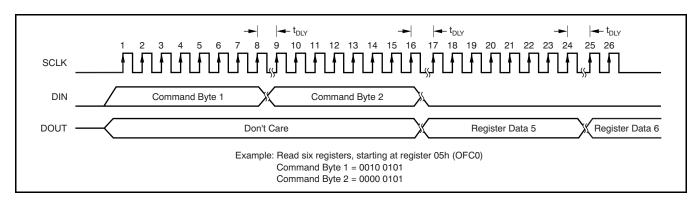
Figure 63. Read Register Data (Table 21 Shows t<sub>DLY</sub>)
