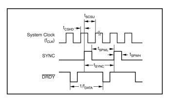
Figure 48. Continuous-Sync Timing with Sync Clock
