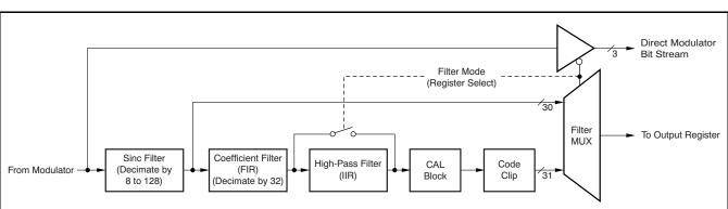
Figure 37. Digital Filter and Output Code Processing
