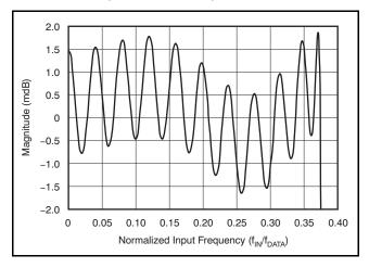
Figure 41. FIR Passband Magnitude Response (f<sub>DATA</sub> = 500Hz)
