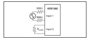
Figure 28. Driving an External Load Through the Mux
