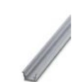
DIN rail, unperforated, Standard profile, width: 35 mm, height: 15 mm, similar to EN 60715, material: Aluminum, uncoated, length: 2000 mm, color: silver
