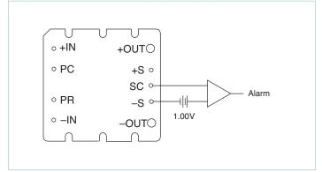
Figure 7 — Secondary-side on-state indicator
