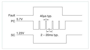
Figure 5 — PC/SC module alarm timing
