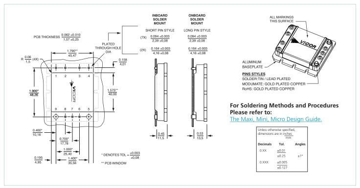
Figure 13 — PCB mounting specifications
