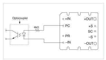
Figure 6 — Isolated on-state indicator
