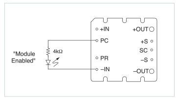
Figure 4 — LED on-state indicator
