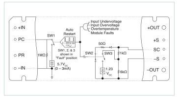
Figure 3 — PC/SC module alarm logic
