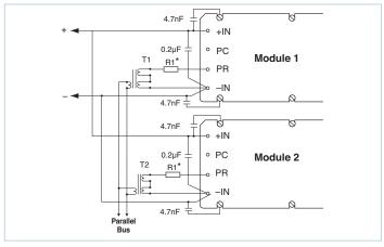
Figure 10 — Transformer-coupled interface
