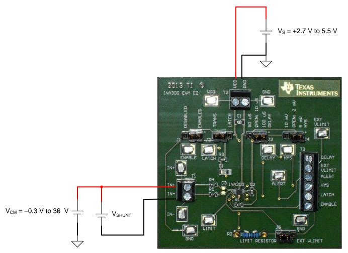
Figure 2. Connecting the INA300EVM with Voltage Sources
