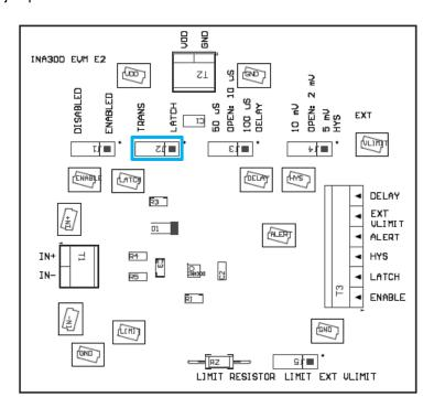
Figure 6. Transparent/Latch Jumper
