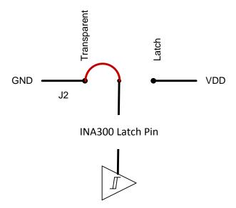
Figure 7. Transparent/Latch Schematic Connections
