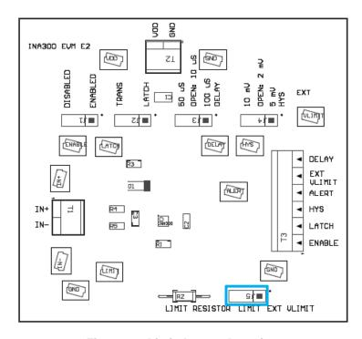
Figure 12. Limit Jumper Location
