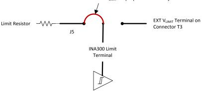
Figure 13. Limit Schematic Connections
