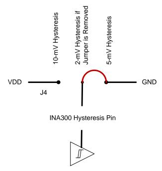
Figure 11. Hysteresis Schematic Connections
