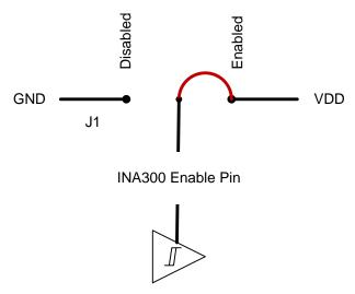
Figure 5. Enable/Disable Schematic Connections
