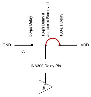
Figure 9. Delay Schematic Connections
