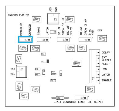
Figure 4. Enable/Disable Jumper Location
