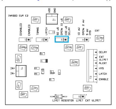
Figure 8. Delay Jumper Location
