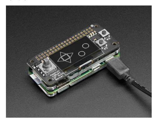
These displays are small, only about 1.3" diagonal, but very readable due to the high contrast of an OLED display. This
