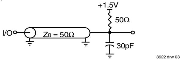
Figure 1. AC Test Load
