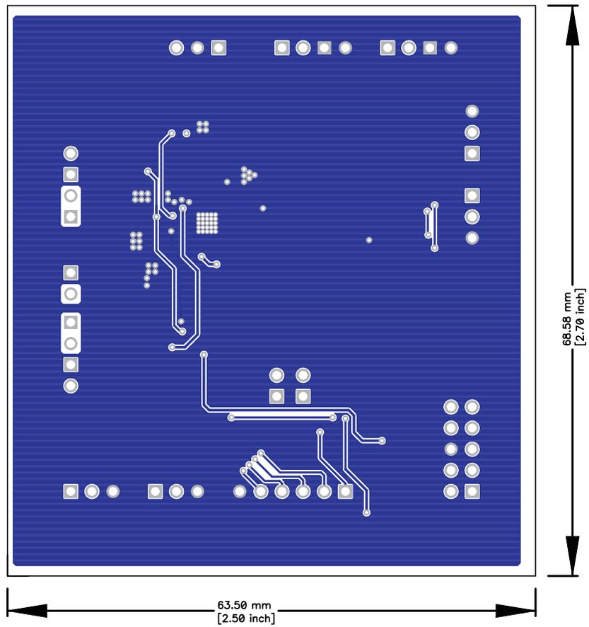
**Figure 10. TPS65721EVM Bottom Copper (X-Ray View )**
