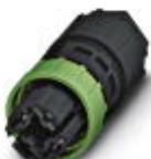
QUICKON-connector, black, 3+PE-pos., 1.0 mm<sup>2</sup> ... 2.5 mm<sup>2</sup>/630 V/20 A, with QUICKON nut, for cables with a diameter of 6 mm ... 10 mm.
