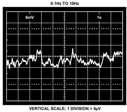
Figure 21. Low Frequency Noise, G = 1 (System Gain = 1000)
