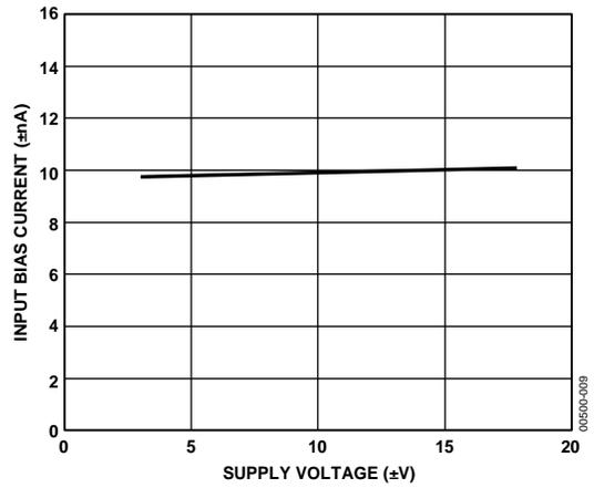
Figure 9. Input Bias Current vs. Supply Voltage
