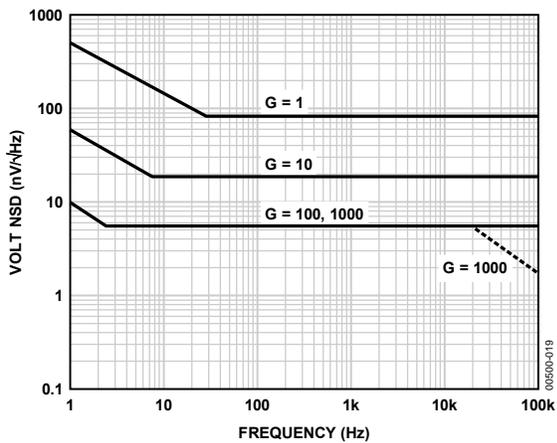
Figure 19. RTI Noise Spectral Density vs. Gain
