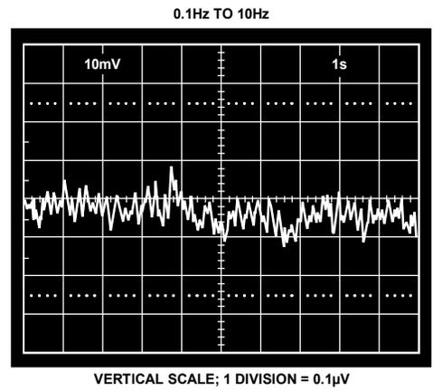
Figure 22. Low Frequency Noise, G = 1000 (System Gain = 100,000)
