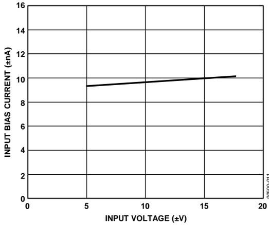
Figure 11. Input Bias Current vs. Input Voltage
