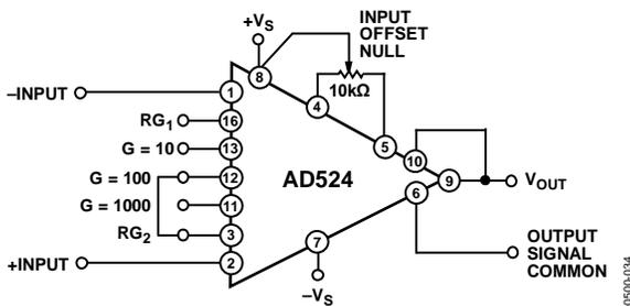
Figure 34. Operating Connections for  $G = 100$
