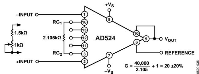
Figure 35. Operating Connections for  $G = 20$
