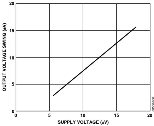
Figure 6. Output Voltage Swing vs. Supply Voltage
