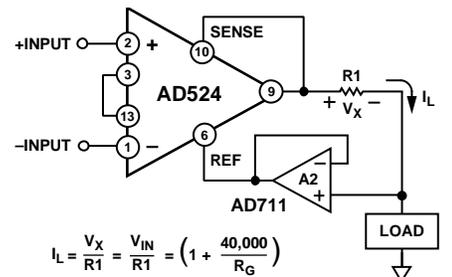
$$I_L = \frac{V_X}{R_1} = \frac{V_{IN}}{R_1} = \left(1 + \frac{40,000}{R_G}\right)$$
