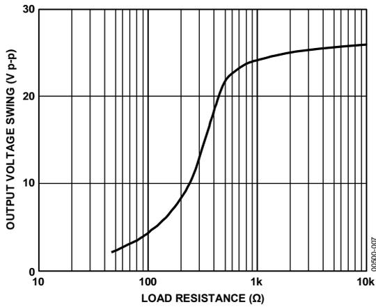
Figure 7. Output Voltage Swing vs. Load Resistance
