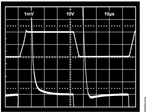
Figure 24. Large Signal Pulse Response and Settling Time, Gain = 1
