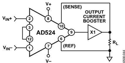
Figure 44. AD524 Instrumentation Amplifier with Output Current Booster
