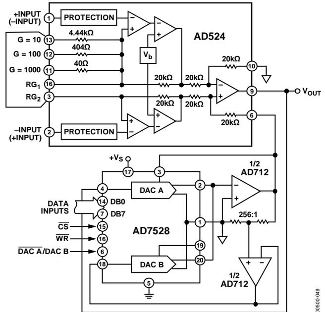
Figure 49. Programmable Output Gain Using a DAC
