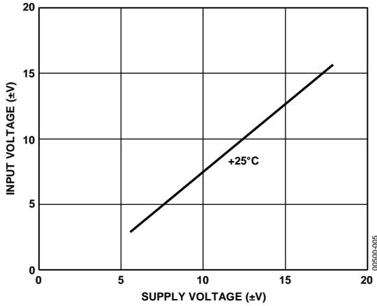
Figure 5. Input Voltage Range vs. Supply Voltage, G = 1
