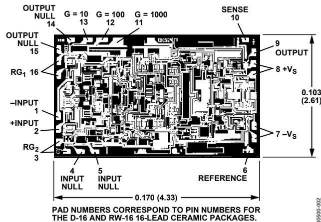
Figure 2. Metallization Photograph
