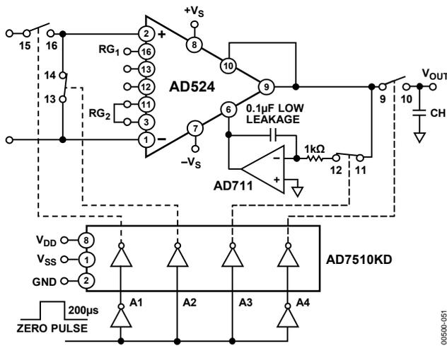
Figure 51. Auto-Zero Circuit
