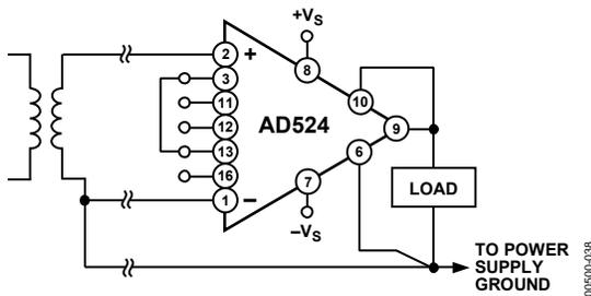
Figure 38. Indirect Ground Returns for Bias Currents—Transformer Coupled
