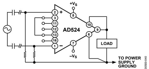
Figure 40. Indirect Ground Returns for Bias Currents—AC-Coupled
