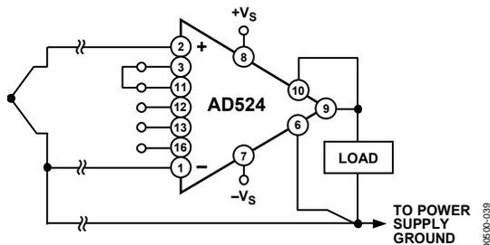
Figure 39. Indirect Ground Returns for Bias Currents—Thermocouple
