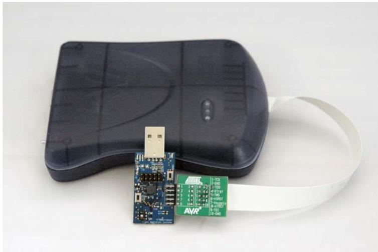
The Flash, EEPROM and all Fuse and Lock Bit options ISP-programmable, can be programmed individually or with the sequential automatic programming option.
