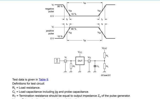
V<sub>EXT</sub> = External voltage for measuring switching times.
