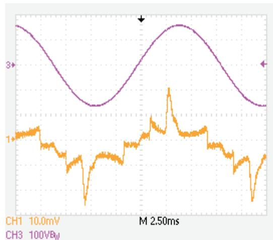
Figure 9. Input AC Voltage and Current, Full Load, No Dimmer
