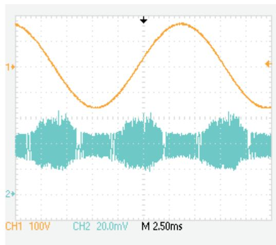
Figure 10. LED Output Voltage Ripple, Full Load, No Dimmer
