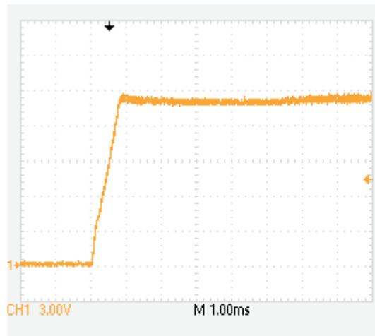
**Figure 8. LED Turn On, Full Load, No Dimmer**
