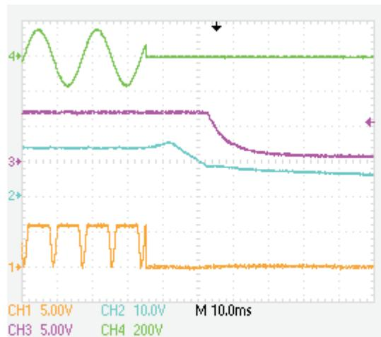
**Figure 17. Turn Off, Full Load, No Dimmer**
