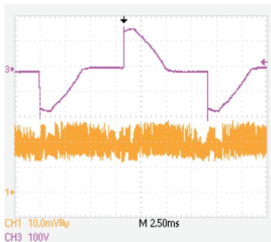
**Figure 12. LED Output Current Ripple, With Dimmer (CH1 = I<sub>LED</sub>, scale = 50 mA/div, CH3 = VIN (115 VAC))**
