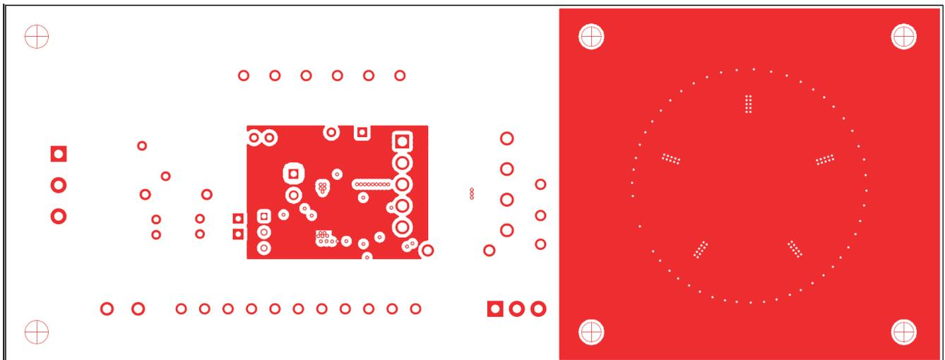
**Figure 26. TPS92070EVM-682 Internal Layer 2 (top view)**
