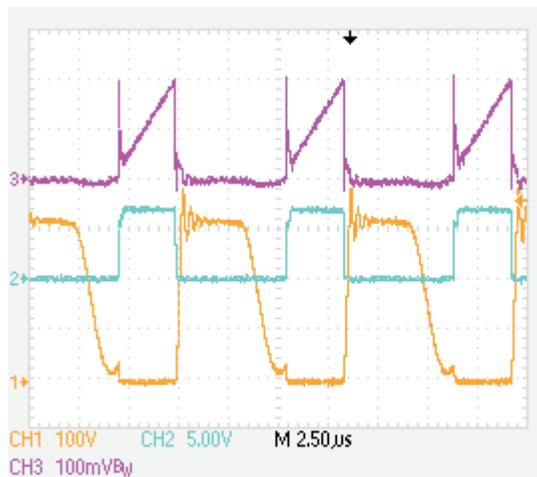
**Figure 13. Switching Waveforms, Full Load, No Dimmer**
