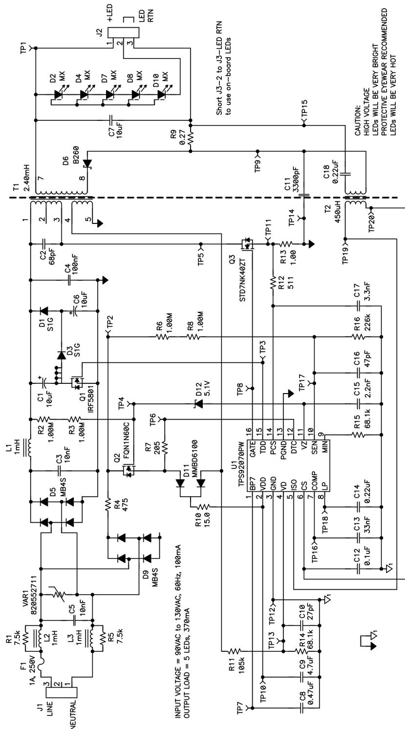
Figure 1. TPS92070EVM-682 Schematic
