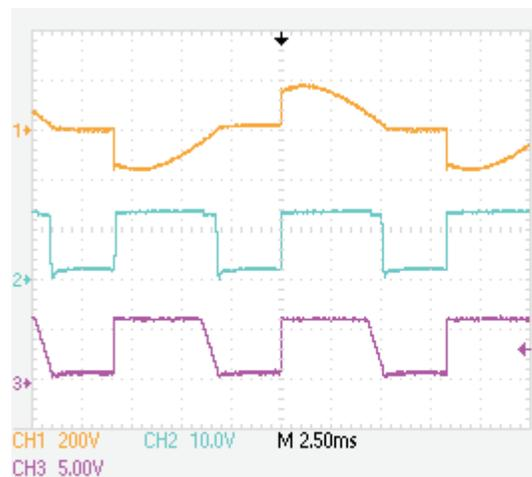
**Figure 18. Dimmer Detection, With Dimmer**
