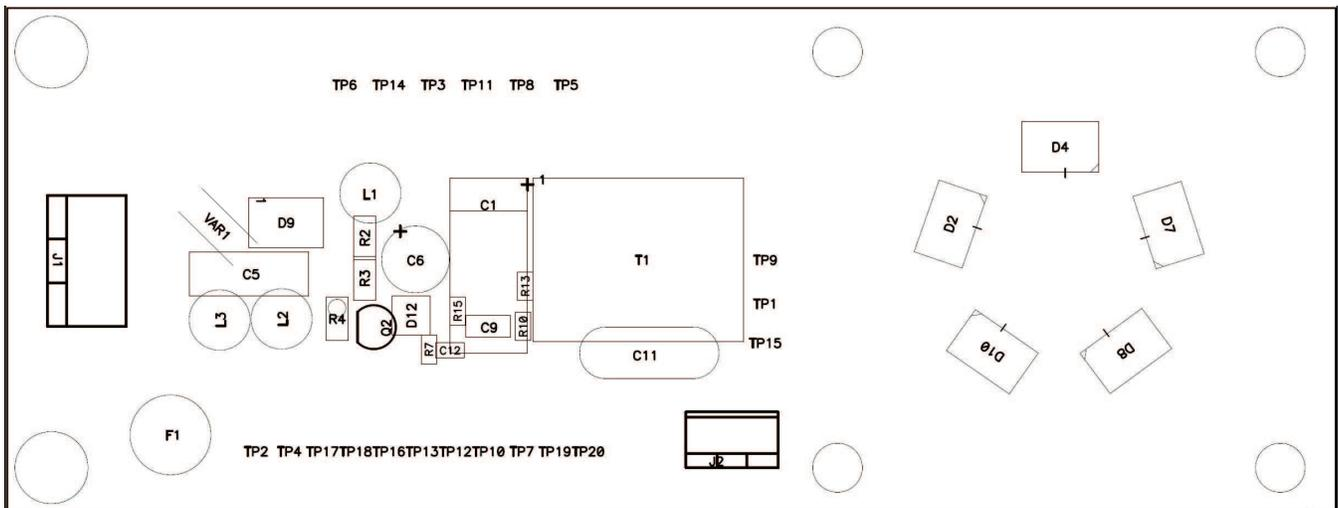
Figure 20. TPS92070EVM-682 Top Layer Assembly Drawing (top view)
