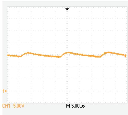
**Figure 11. LED Output Current Ripple, Full Load, No Dimmer (CH1 = VIN (115 VAC), CH2 = I<sub>LED</sub>, scale = 200 mA/div)**
