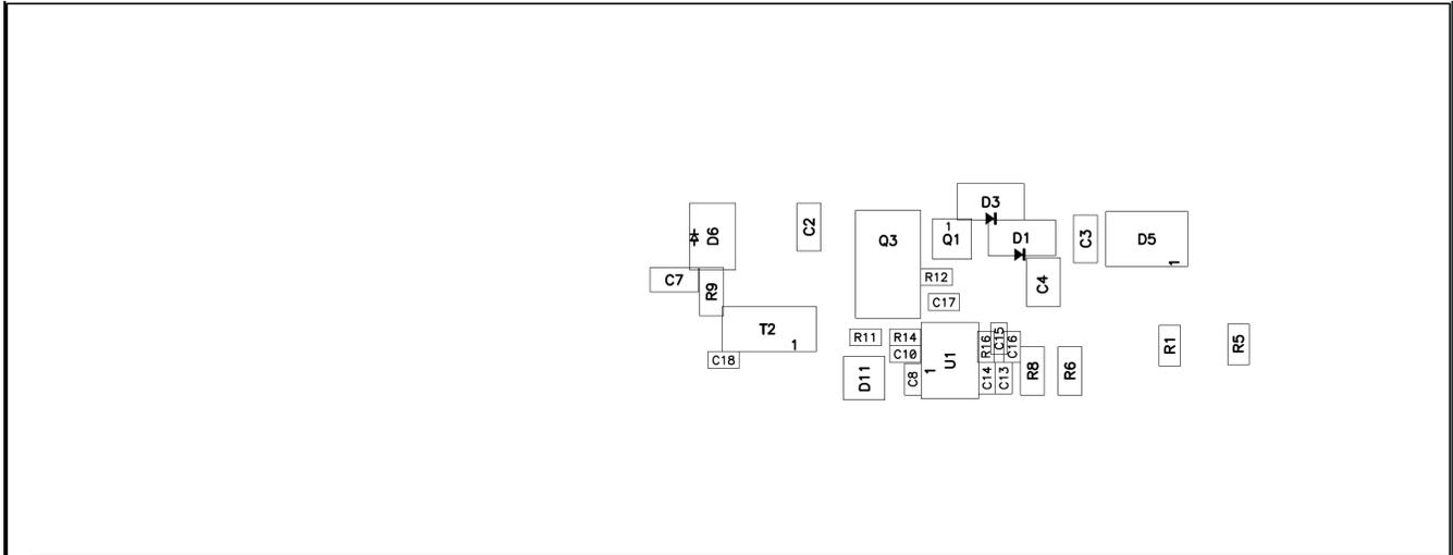
**Figure 23. TPS92070EVM-682 Bottom Layer Assembly Drawing (bottom view)**
