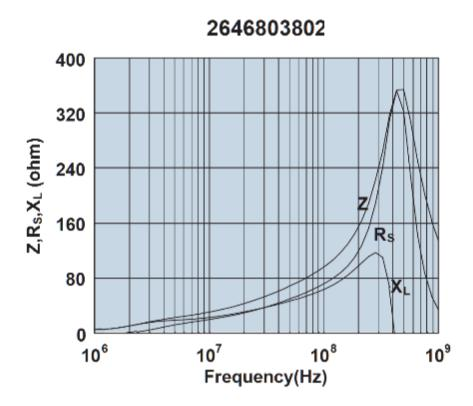
Impedance, reactance, and resistance vs. frequency.
