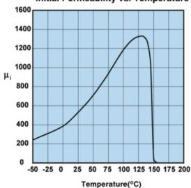
Measured on a 17/10/6mm toroid at 100kHz.
