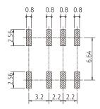
PC board mounting pad layout (TOP VIEW)
