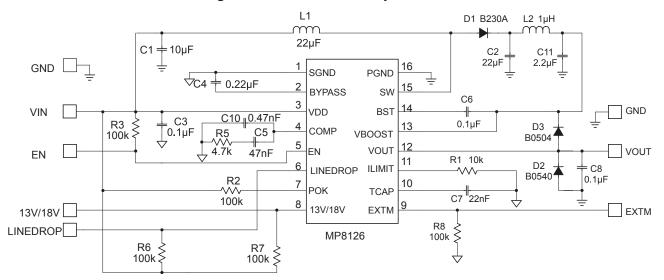
Figure 4: Detailed Application Schematic
