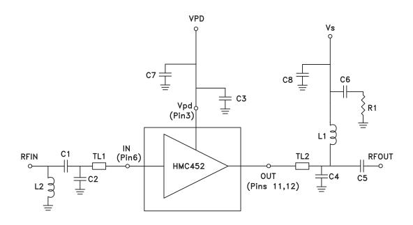
Note: C2, C3 and C4 should be placed as close to pins as possible.
