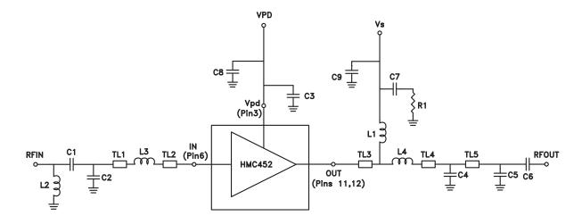
Note: C3 should be placed as close to pins as possible.
