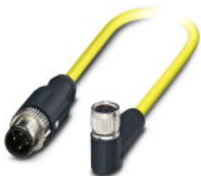
Sensor/actuator cable, 4-position, PVC, yellow, shielded, Plug straight M12 SPEEDCON, coding: A, on Socket angled M8, cable length: 1.5 m
