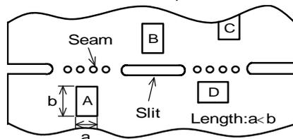
Products (A,B,C,D) shall be located carefully so that products are not subject to the mechanical stress due to warping the board. Because they may be subjected the mechanical stress in order of  $A > C > B \cong D$ .
