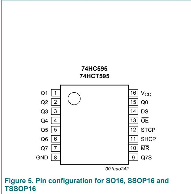
Figure 5. Pin configuration for SO16, SSOP16 and TSSOP16
