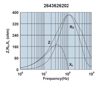
Impedance, reactance, and resistance vs. frequency.
