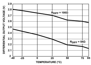
FIGURE 10. DRIVER DIFFERENTIAL OUTPUT VOLTAGE vs TEMPERATURE
