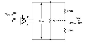
FIGURE 4A.  $V_{OD}$  AND  $V_{OC}$
