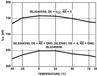
FIGURE 12. SUPPLY CURRENT vs TEMPERATURE
