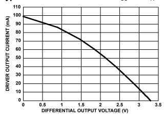
FIGURE 9. DRIVER OUTPUT CURRENT VS DIFFERENTIAL OUTPUT VOLTAGE
