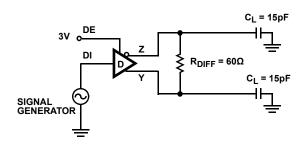
FIGURE 5A. DIFFERENTIAL TEST CIRCUIT
