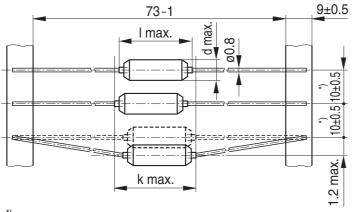
$<sup>^{*)}</sup>$  Tolerance over 10 spacings ±2 mm
