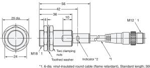
\*1. 6-dia. vinyl-insulated round cable (flame retardant), Standard length; 300 mm \*2. Operation indicator (red/green) Setting indicator (green)
