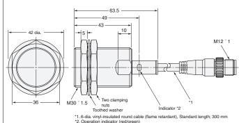
\*1.6-dia. vinyl-insulated round cable (flame retardant), Standard length; 300 mm
