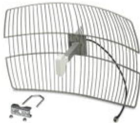
Parabolic antenna, IP65 degree of protection, 19 dBi gain, linear vertical, N (female) connection, impedance 50 Ω, apex angle h/v 17°/11°
