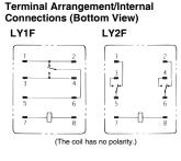
**Note:** The figures and dimensions depicted here are for the LY1F. The LY2F is also conforms to these measurements.
