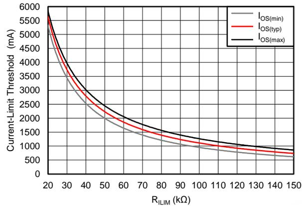
**Figure 16. Current-Limit Threshold versus R<sub>(ILIM)</sub>**
