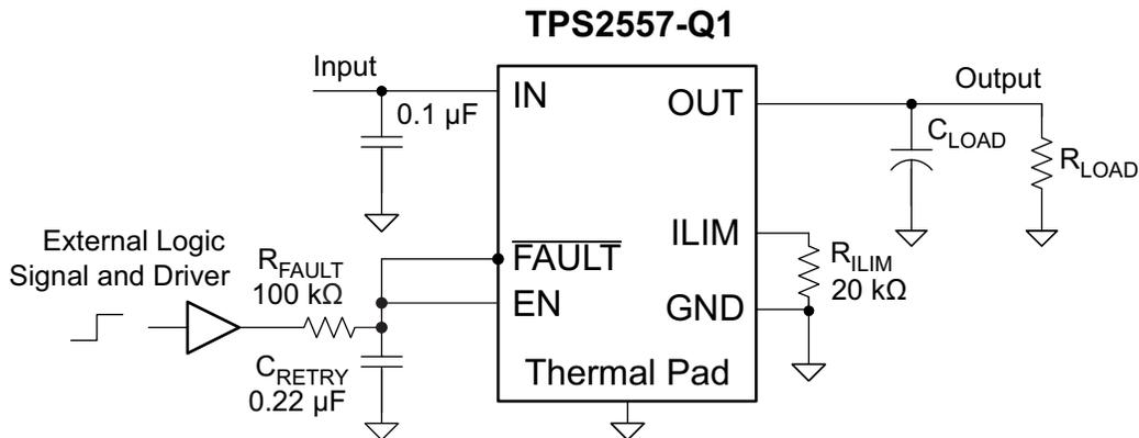
Figure 13. Auto-Retry Functionality With External EN Signal
