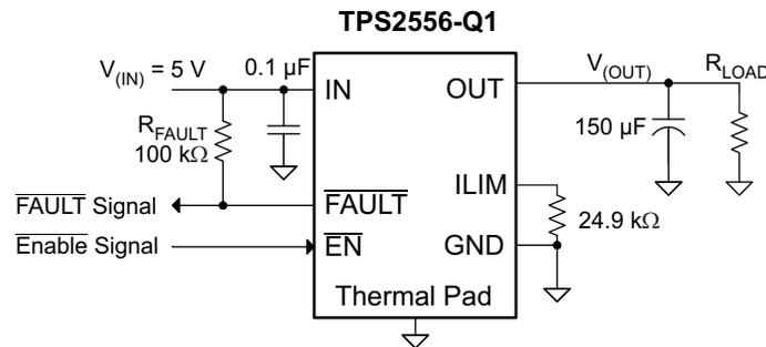
**Figure 15. Application Schematic for Current Limit, TPS2556-Q1**
