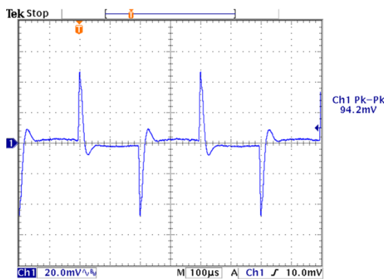
Figure 9 Transient Response with Regulation set to 0 mV/A
