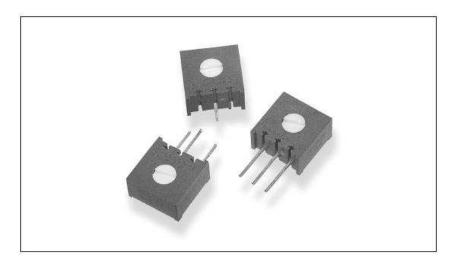
These long established 10mm square, single turn potentiometers will meet wide range of industrial and professional applications. Cermet element technology ensures stability and reliability. This P.C.B. mounted package has easy top or side adjustment, or finger adjust styles. All components are sealed to withstand printed circuit board washing solvents.
