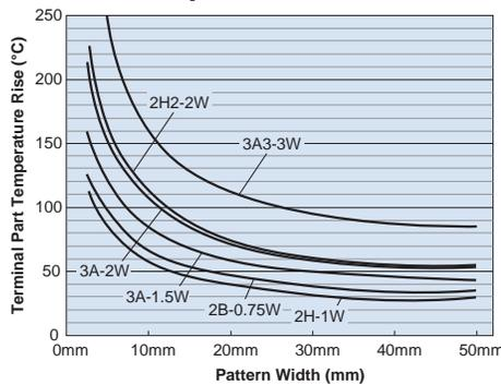
Room Temperature 25°C PCB: FR-4 t=1.6mm Cu foil thickness=35μm
