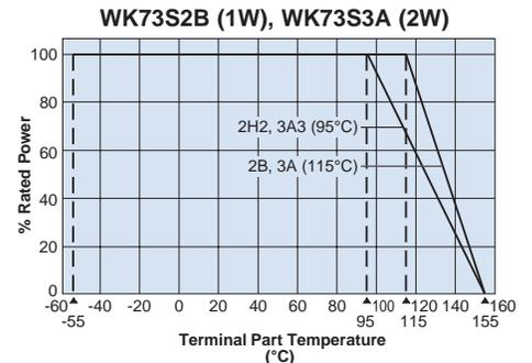
If you want to use at rated power (\*1), use derating curves based on the terminal part temperature on the right side graph.
