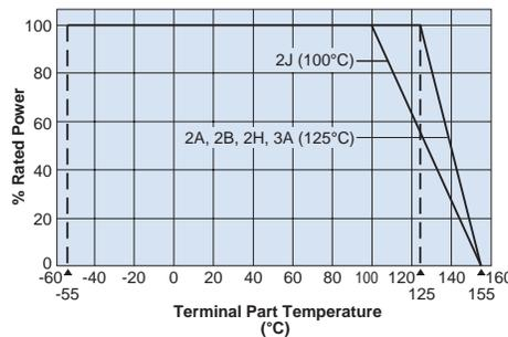
For resistors operated terminal temperature of described for each size or above, a power rating shall be derated in accordance with the derating curve above. Please refer to "Introduction of the derating curve based on the terminal part temperature" in the beginning of our catalog before use.
