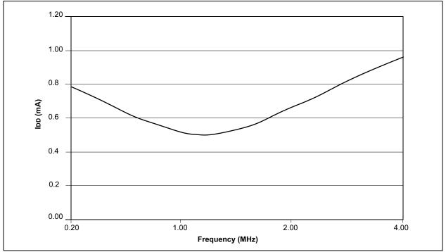
FIGURE 13-1: IDD VS. FREQUENCY (XT MODE, VDD = 5.5V)
