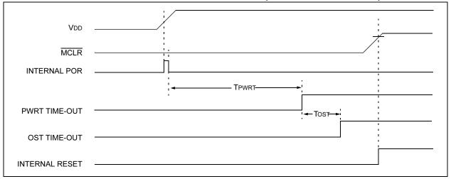
FIGURE 9-10: TIME-OUT SEQUENCE ON POWER-UP (MCLR TIED TO VDD)
