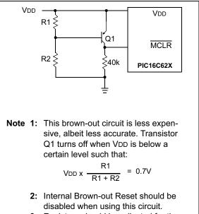
**3:** Resistors should be adjusted for the characteristics of the transistor.
