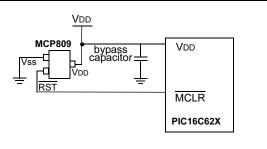
This brown-out protection circuit employs Microchip Technology's MCP809 microcontroller supervisor. The MCP8XX and MCP1XX families of supervisors provide push-pull and open collector outputs with both high and low active RESET pins. There are 7 different trip point selections to accommodate 5V and 3V systems.
