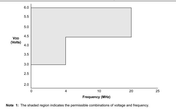
**2:** The maximum rated speed of the part limits the permissible combinations of voltage and frequency. Please reference the Product Identification System section for the maximum rated speed of the parts.
