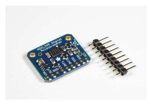
The ADXL345 is a low-power, 3-axis MEMS accelerometer modules with both I2C and SPI interfaces. The Adafruit Breakout boards for these modules feature on-board 3.3v voltage regulation and level shifting which makes them simple to interface with 5v microcontrollers such as the Arduino.
