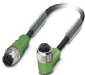
Sensor/actuator cable, 4-position, PUR halogen-free, black-gray RAL 7021, Plug straight M12, A-coded, on Socket angled M12, A-coded, cable length: 10 m
