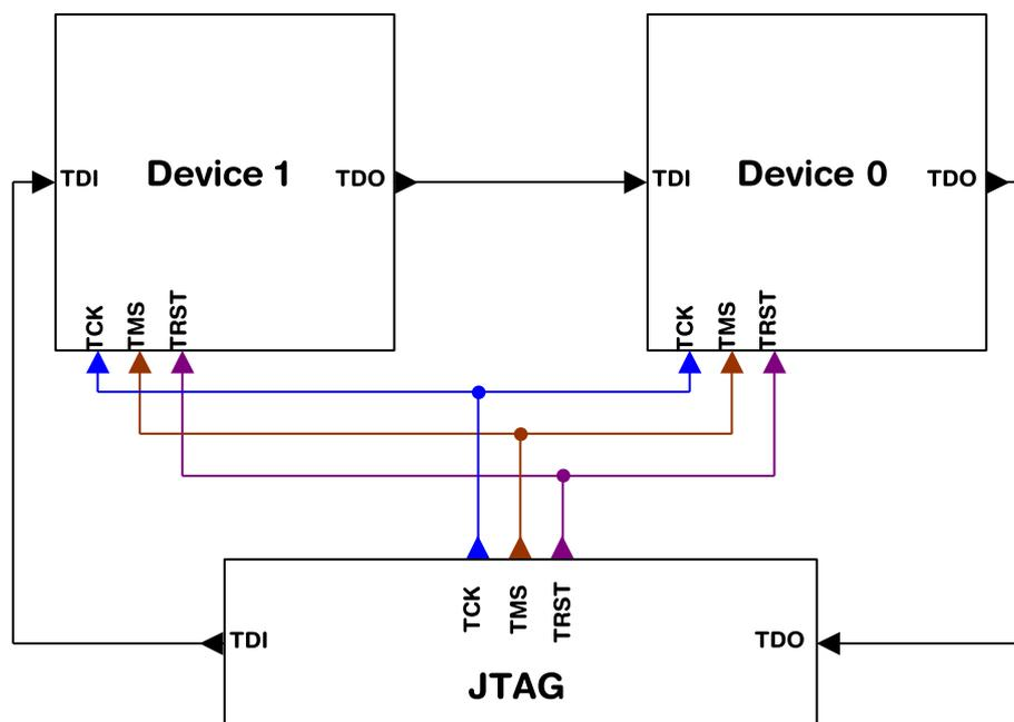
Currently, up to 8 devices in the scan chain are supported. One or more of these devices can be CPU cores; the other devices can be of any other type but need to comply with the JTAG standard.
