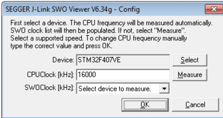
When running in normal mode J-Link SWO Viewer automatically performs the necessary initialization to enable SWO output on the target, in GDB Server mode the initialization has to be done by the debugger. Should you have a target connection already open e.g. a debug session in your IDE we recommend defining the parameters device name, CPU clock frequency and SWO clock frequency via CL to avoid connection errors.
