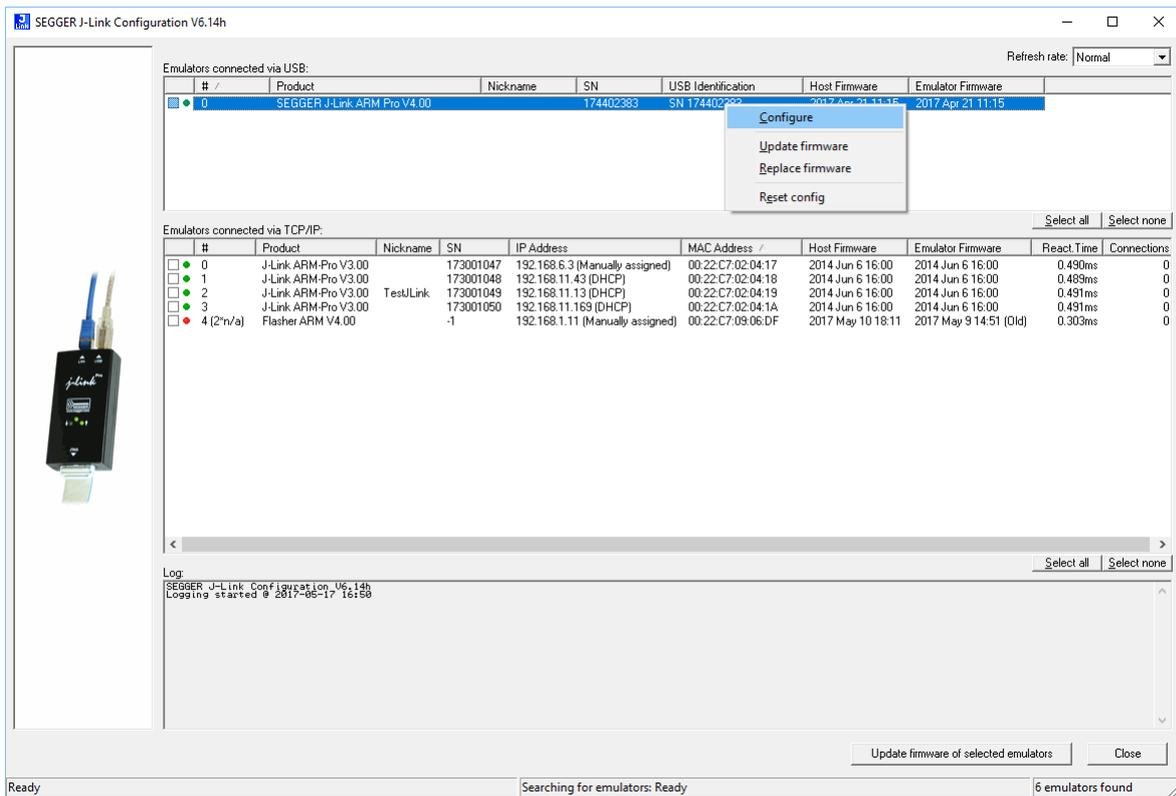
In order to configure an old J-Link, which uses the old USB 0 - 3 USB identification method, to use the new USB identification method (reporting the real serial number) simply select "Real SN" as USB identification method and click the OK button. The same dialog also allows configuration of the IP settings of the connected J-Link if it supports the Ethernet interface.
