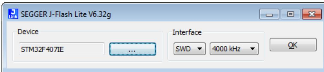
The main window of J-Flash Lite only consists of a few dialog elements that allow programming of the target:
