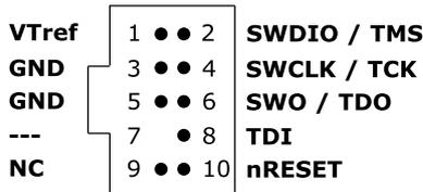
Some target boards only provide a 9-pin JTAG/SWD connector for Cortex-M. or these devices SEGGER provides a 20-pin -> 9-pin Cortex-M adapter.
