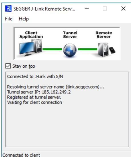
*J-Link Remote Server: Connected to SEGGER tunnel server*
