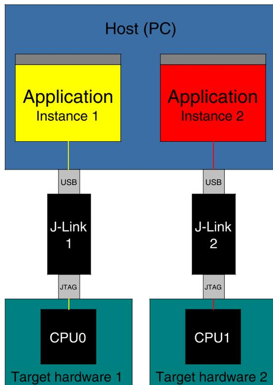
Older J-Links may report USB0-3 instead of unique serial number when enumerating via USB. For these J-Links, we recommend to re-configure them to use the new enumeration method (report real serial number) since the USB0-3 behavior is obsolete.
