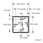
For the make contact (2x87), pin 87a = 87; for the double make contact, pin 87a = 87b.
