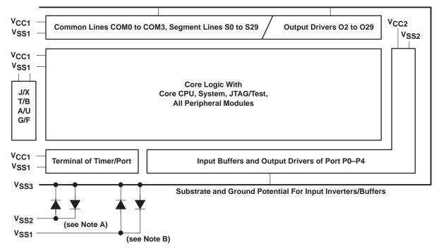
NOTES: A. Ground potential for all port output drivers and input terminals, excluding first inverter/buffer
