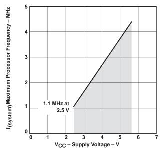
Figure 3. Processor Frequency vs Supply Voltage
