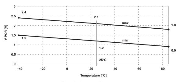
Figure 5. V<sub>(POR)</sub> vs Temperature
