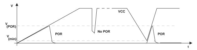
Figure 4. Power-On Reset (POR) vs Supply Voltage
