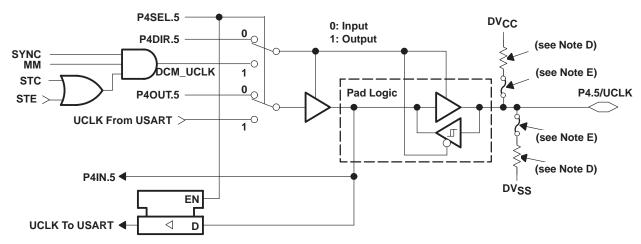
Figure 17. Port P4, P4.5, Input/Output With Schmitt-Trigger
