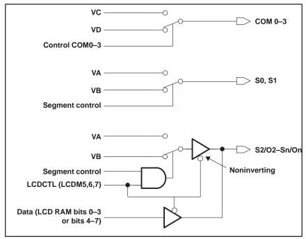
LCD OUTPUT (COM0-4, Sn, Sn/On)
