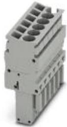
Plug, Connection method: Spring-cage connection, Number of positions: 6, Cross section: 0.08 mm<sup>2</sup> - 4 mm<sup>2</sup>, AWG: 28 - 12, Width: 31.2 mm, Height: 39 mm, Color: gray
