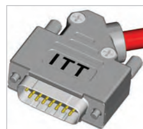
Assemble the other half (screwing force: 100-120 Ncm)
