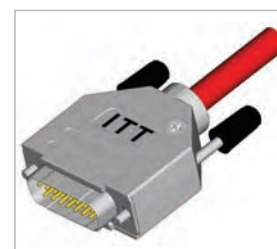
Assemble the other half (screwing force: 100-120 Ncm)
