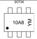
10A8 = Product Type Marking Code YM = Date Code Marking Y or  $\overline{Y}$  = Year (ex: C = 2015) M or  $\overline{M}$  = Month (ex: 9 = September)
