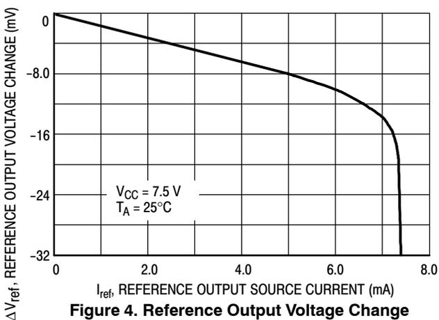
**Figure 4. Reference Output Voltage Change versus Source Current**
