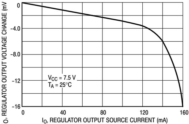
**Figure 2. Regulator Output Voltage Change versus Source Current**
