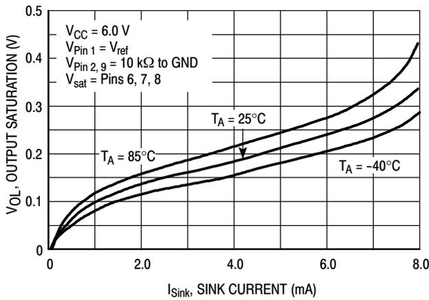
**Figure 8. Comparator Output Saturation versus Sink Current**
