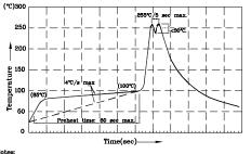
Notes: 1.Recommend pre-heat temperature of 105°C or less (as me thermocouple attached to the LED pins) prior to immersion wave with a maximum solder bath temperature of 260°C 2.Peak wave soldering temperature between 245°C ~ 255°C for a solution of the solution of max)
