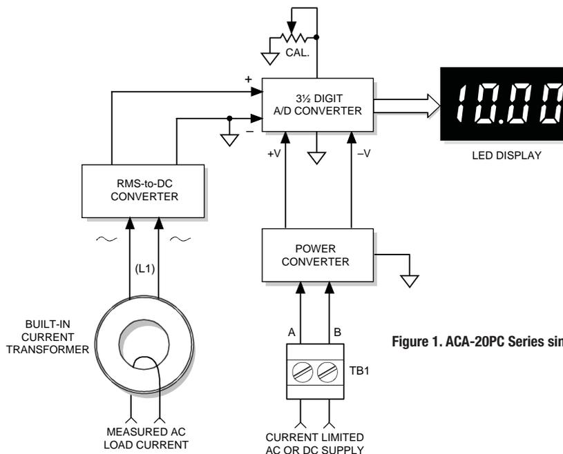
Figure 1. ACA-20PC Series simplified schematic
