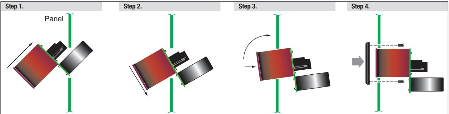
Figure 2. Panel Installation
