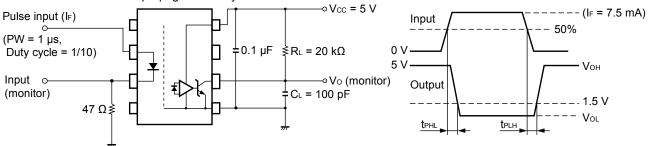
Remark C<sub>L</sub> includes probe and stray wiring capacitance.
