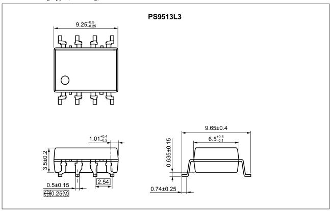
• Lead Bending Type For Long Creepage Distance
