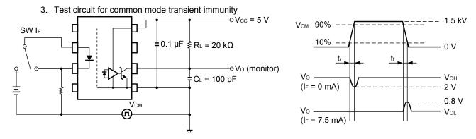
Remark C<sub>L</sub> includes probe and stray wiring capacitance.
