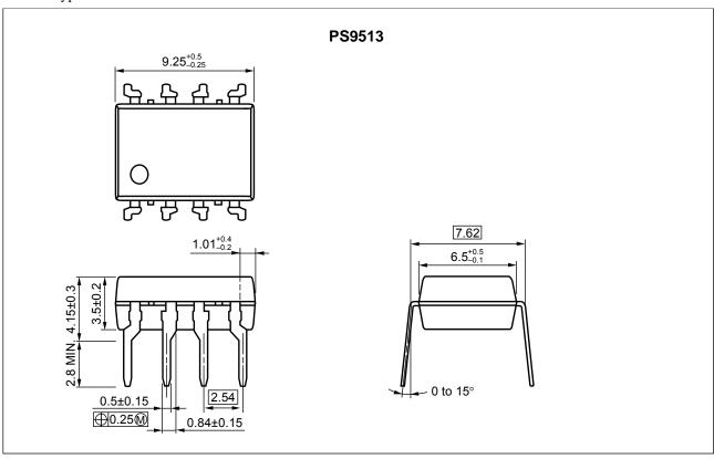
• Lead Bending Type (Gull-wing) For Surface Mount
