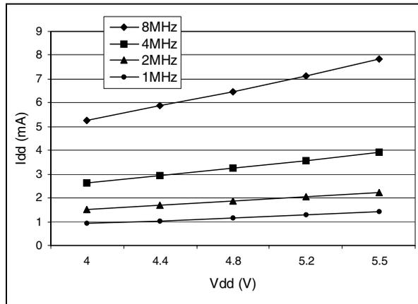
**Figure 63. Typical  $I_{DD}$  in WAIT mode**
