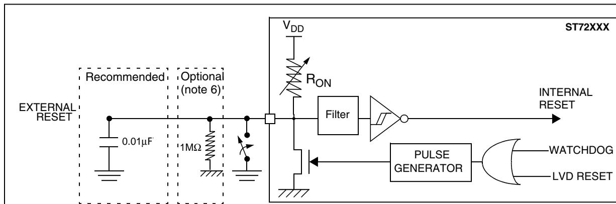
Figure 78.  $\overline{\text{RESET}}$  pin protection when LVD is disabled. 1)2)3)4)
