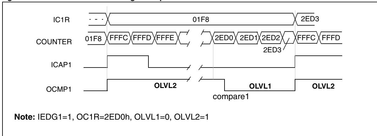
Figure 45. Pulse Width Modulation Mode Timing Example with 2 Output Compare Functions
