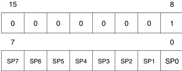
The Stack Pointer is a 16-bit register which is always pointing to the next free location in the stack. It is then decremented after data has been pushed onto the stack and incremented before data is popped from the stack (see Figure 9).
