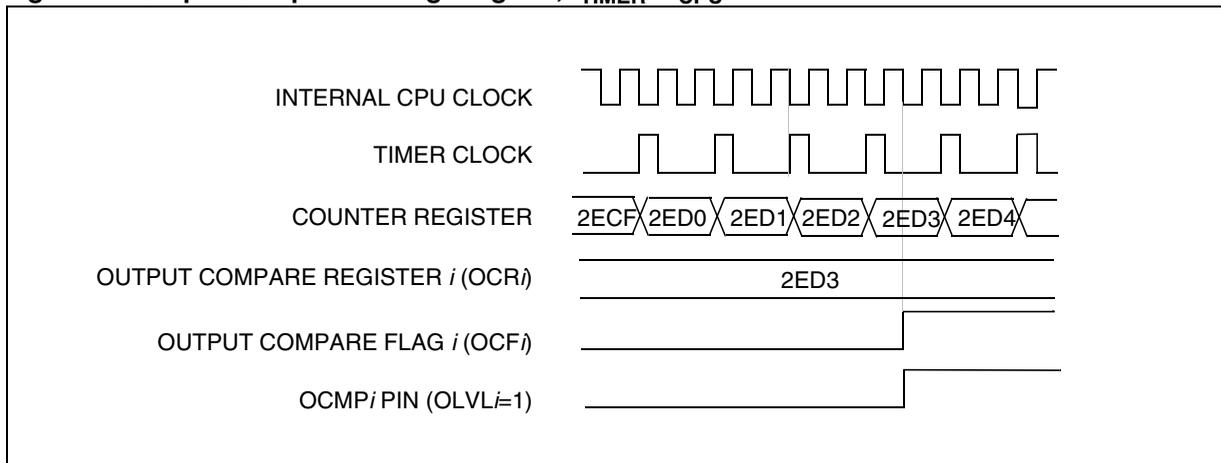
Figure 43. Output Compare Timing Diagram,  $f_{TIMER} = f_{CPU}/4$
