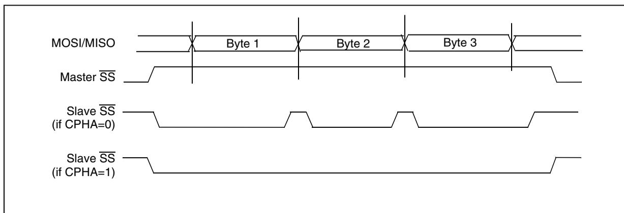
**Figure 49. Hardware/Software Slave Select Management**
