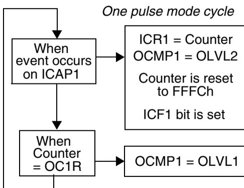
Then, on a valid event on the ICAP1 pin, the counter is initialized to FFFCh and OLVL2 bit is loaded on the OCMP1 pin, the ICF1 bit is set and the value FFFDh is loaded in the IC1R register.
