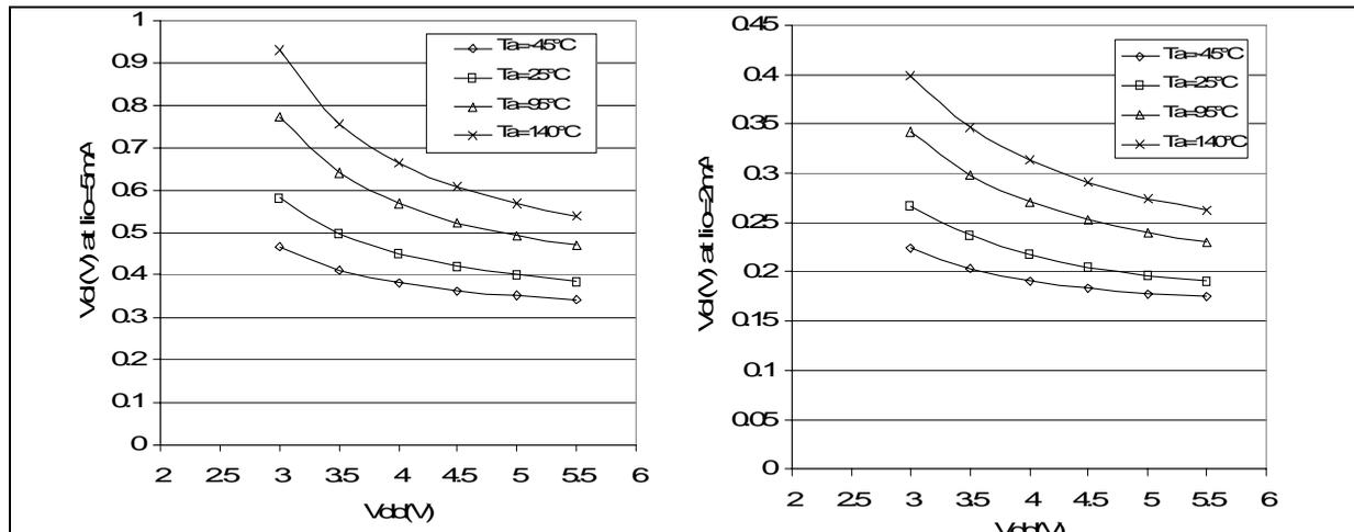
Figure 75. Typical  $V_{OL}$  vs.  $V_{DD}$  (high-sink ports)
