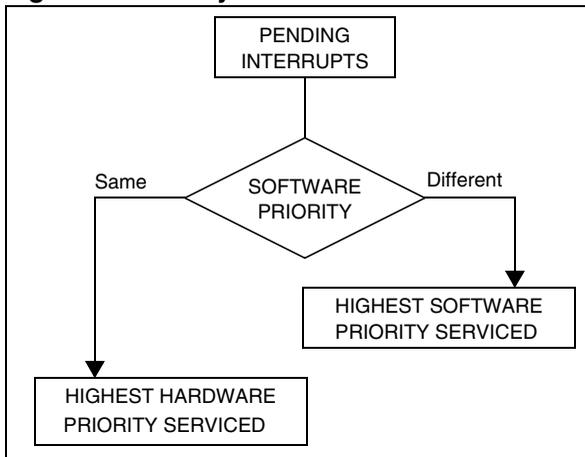
When an interrupt request is not serviced immediately, it is latched and then processed when its software priority combined with the hardware priority becomes the highest one.
