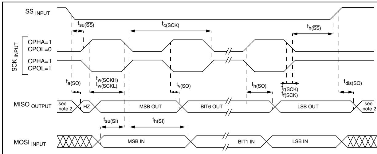
Figure 82. SPI Master Timing Diagram <sup>1)</sup>
