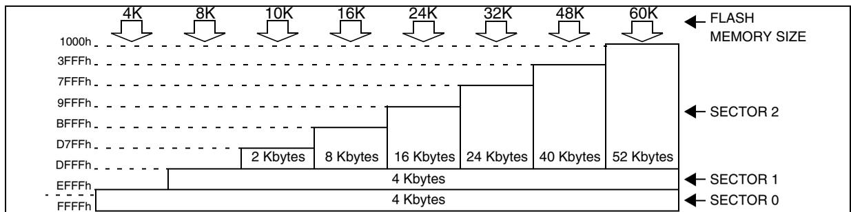
Depending on the overall Flash memory size in the microcontroller device, there are up to three user sectors (see Table 3). Each of these sectors can be erased independently to avoid unnecessary erasing of the whole Flash memory when only a partial erasing is required.
