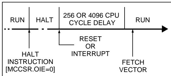
Figure 28. HALT Mode Flow-chart
