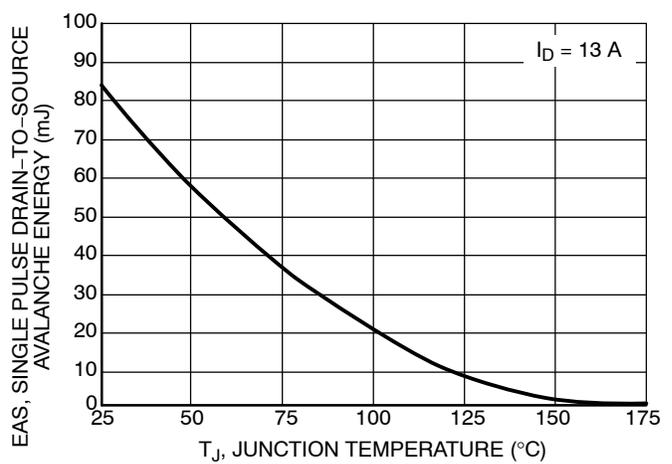
Figure 12. Maximum Avalanche Energy vs. Starting Junction Temperature
