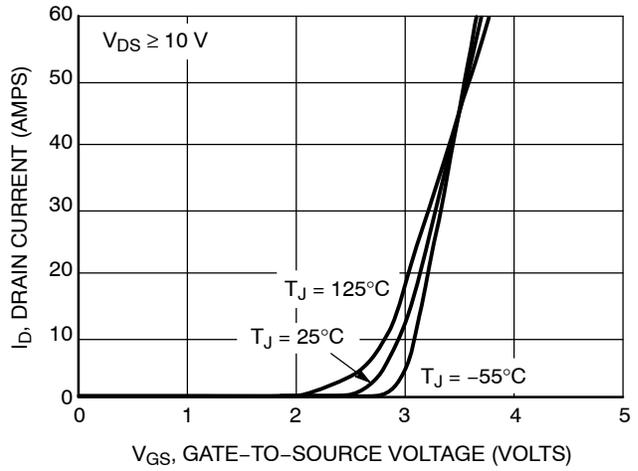
Figure 2. Transfer Characteristics
