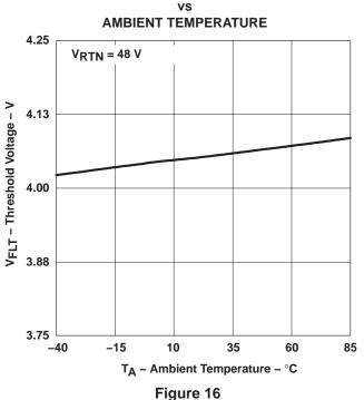
**FAULT LATCH THRESHOLD**
