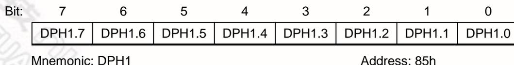
This is the high byte of the new additional 16-bit data pointer that has been added to the W77C032. The user can switch between DPL, DPH and DPL1, DPH1 simply by setting register DPS = 1. The instructions that use DPTR will now access DPL1 and DPH1 in place of DPL and DPH. If they are not required they can be used as conventional register locations by the user.
