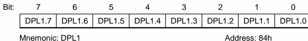
This is the low byte of the new additional 16-bit data pointer that has been added to the W77C032. The user can switch between DPL, DPH and DPL1, DPH1 simply by setting register DPS = 1. The instructions that use DPTR will now access DPL1 and DPH1 in place of DPL and DPH. If they are not required they can be used as conventional register locations by the user.
