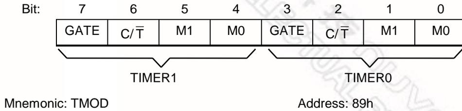
GATE: Gating control: When this bit is set, Timer/counter x is enabled only while  $\overline{\text{INTx}}$  pin is high and TRx control bit is set. When cleared, Timer x is enabled whenever TRx control bit is set.
