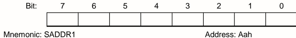
SADDR1: The SADDR1 should be programmed to the given or broadcast address for serial port 1 to which the slave processor is designated.
