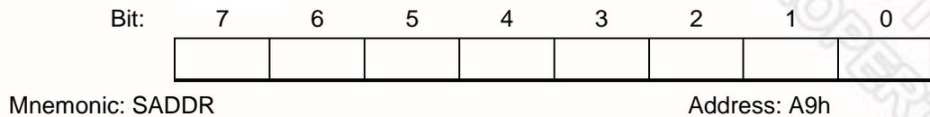
SADDR: The SADDR should be programmed to the given or broadcast address for serial port 0 to which the slave processor is designated.
