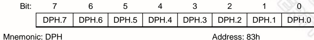
This is the high byte of the standard 8052 16-bit data pointer.
