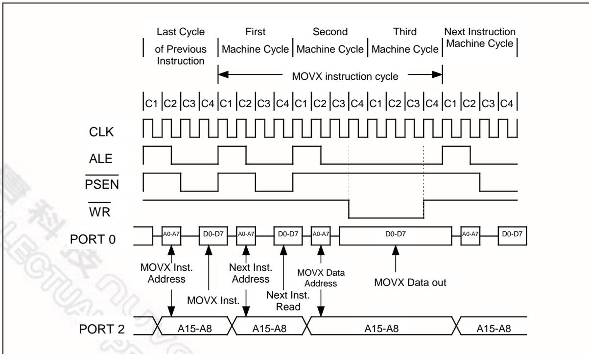
Figure 9: Data Memory Write with Stretch Value = 1
