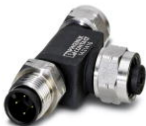
Bus system T-connector, 5-position, unshielded, Plug straight M12, A-coded, on Socket straight M12, A-coded, PIN 2+4 bridged and Socket straight M12, A-coded, PIN 2+4 bridged, Special wiring
